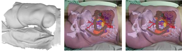
Fig. 3. Results with a human patient in a live operating room. The RGBD scan (left), rigid registration (middle) and deformable registration (right).
